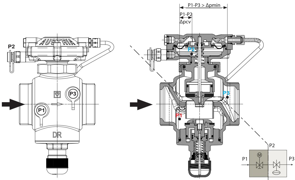
**$k_v$  - values of the control valve in the PIBCV (test points P1 - P2)**
