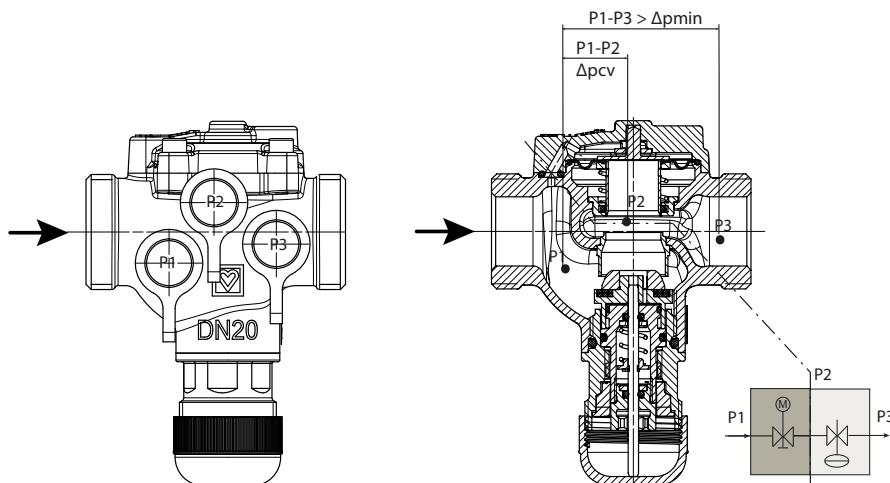
**$k_v$  - values of the control valve in the PIBCV (quick test point P1 - P2)**
