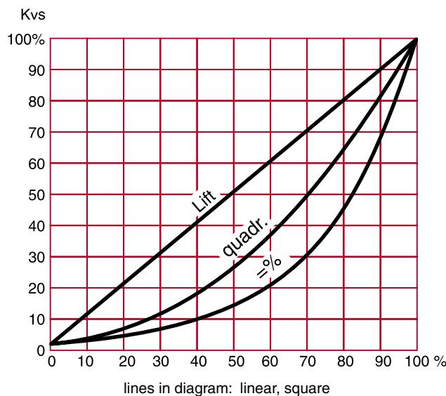
Linear valve characteristic could be changed by using the valve drive 1 7712 11 with fitted DIP switches.
